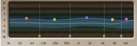
The MultiBand graph is like an EQ graph showing Amplitude in the Y-axis and Frequency in X-axis. In the Middle of the graph resides the DynamicLine<sup>TM</sup> that shows the per band gain adjustment as it happens within the Range, represented by the Bluish highlight. Beneath the graph there are the 4 Crossover frequency markers and on the graph there are 5 markers that allow you to set the gain of the band by dragging up and or down and the band's width by dragging sideways.
